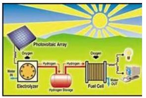
Figure 3: Block Diagram showing generation of solar energy.
